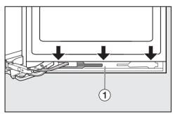
Remove panel ① from the soft-close mechanism by inserting a flat-bladed screwdriver into the gap from above and easing it off bit by bit. Take care not to damage the door seal.
